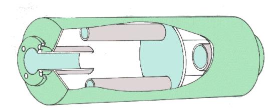
These silencers are designed on the reactive principle with twin chambers in which the exhaust gases are mixed and smoothed, thus absorbing a high proportion of the acoustic energy without causing excessive back pressure.
