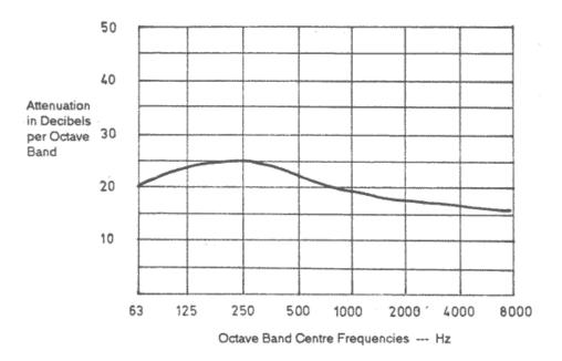
The above graph is based on simplified theoretical considerations and extrapolated from various noise tests. The actual noise reduction obtained on any particular installation will depend upon the power and type of the noise source, the local environment and the selection of the correct size of silencer for that engine.
