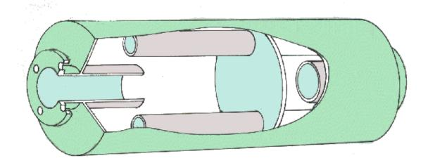
These silencers are designed on the reactive principle with twin chambers in which the exhaust gases are mixed and smoothed, thus absorbing a high proportion of the acoustic energy without causing excessive back pressure.
