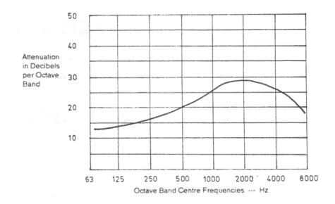
The above graph is based on simplified theoretical considerations and extrapolated from various noise tests. The actual noise reduction obtained on any particular installation will depend upon the power and type of the noise source, the local environment and the selection of the correct size of silencer for that engine.
