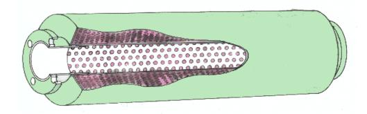
These silencers can be used on either diesel exhausts or air systems. They are constructed on the sound absorption principle. The gases pass through a centre duct surrounded by sound absorbent material and the minimum resistance is offered to the gas flow.
